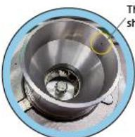
7. Reinstall the upper burr holder in the corresponding groove.
