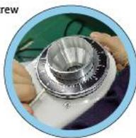
8. Re-screw the adjusting plate counterclockwise. Pay attention to screw tightening.
