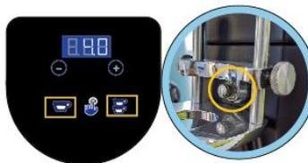
In the standard mode, the single/double dose button is lighted. Press the single/double dose button, then touch and release the micro switch to start grinding. Or Vice Versa.
