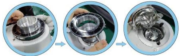
2. Press down the thimble piece and turn the adjusting handle clockwise at the same time, remove the adjusting plate, and remove the upper burr holder.
