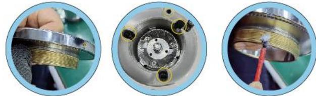
4. Clean the copper thread on the adjusting plate with soft cloth.
