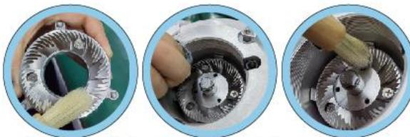
4. Use a cleaning brush and soft cloth to thoroughly clean the grinding blades, threads and the entire grinding system. It is recommended to use a small metal brush on the threaded part of the device.
