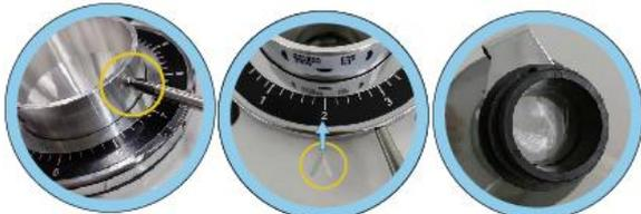
1. Clear the coffee beans in the hopper, close the bean baffle, unscrew the locking screw to remove the bean hopper.
