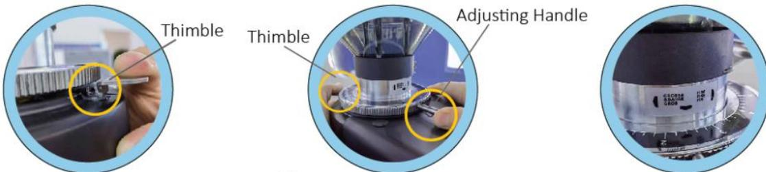
① Press the thimble that fixes the adjusting plate, so that the adjusting plate can be rotated;
