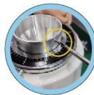
9. Reinstall the locking screw on the upper burr holder.
