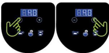
Long press the "+" or "-" key until the buzzer long beeps once, the grinding mode is switched between the standard mode and the preselected mode.
